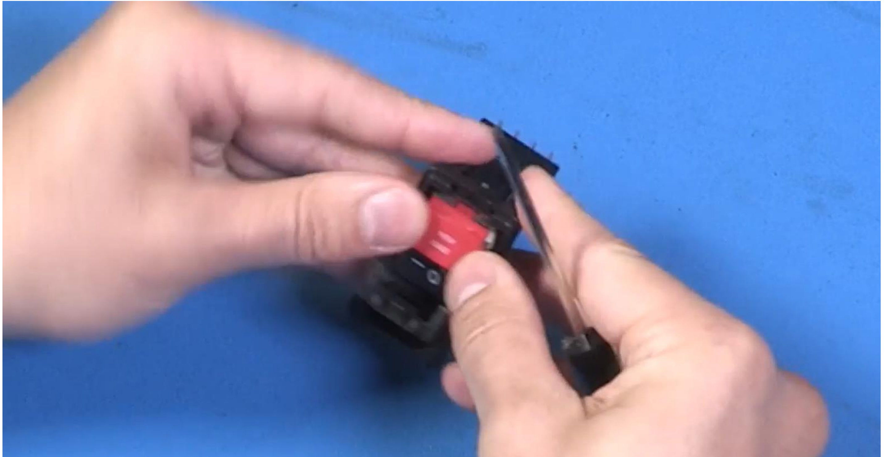
Figure 8. Detail of Fuse Installed (AC Model)
