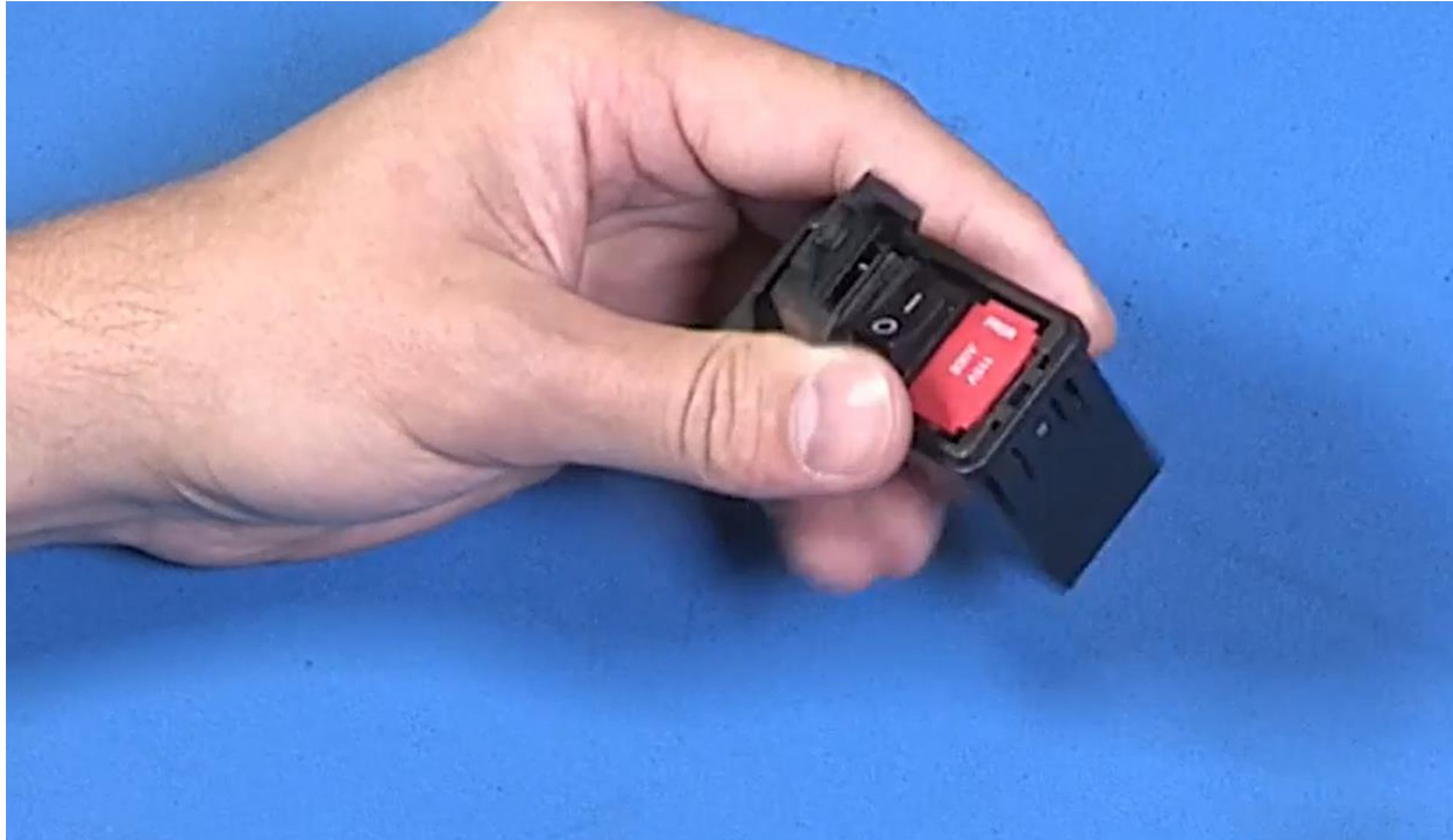
Figure 6. Opened Fuse Housing (AC Model)
