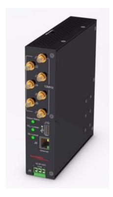
Brandywine's RFS-700D is a miniaturized Rubidium Frequency Reference in a compact ruggedized package designed for mounting on a DIN rail system. The RFS-700D is capable of outputting 7x 10MHz frequency reference with low phase noise.
