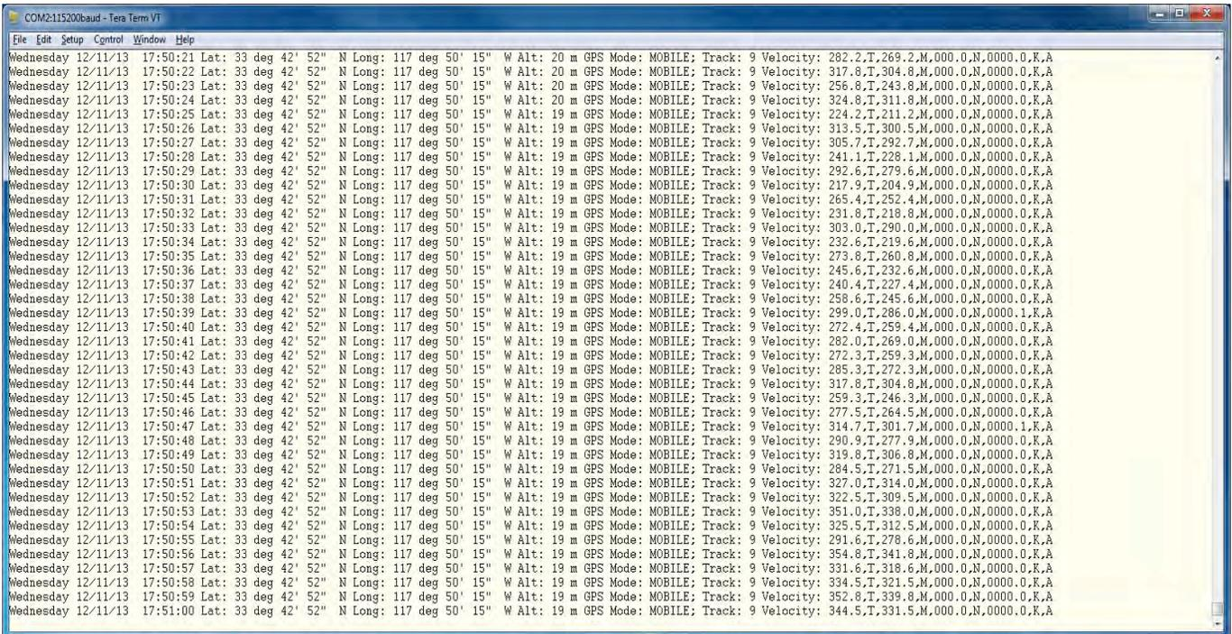
Figure 19 - Serial Time, Position and Velocity output.
