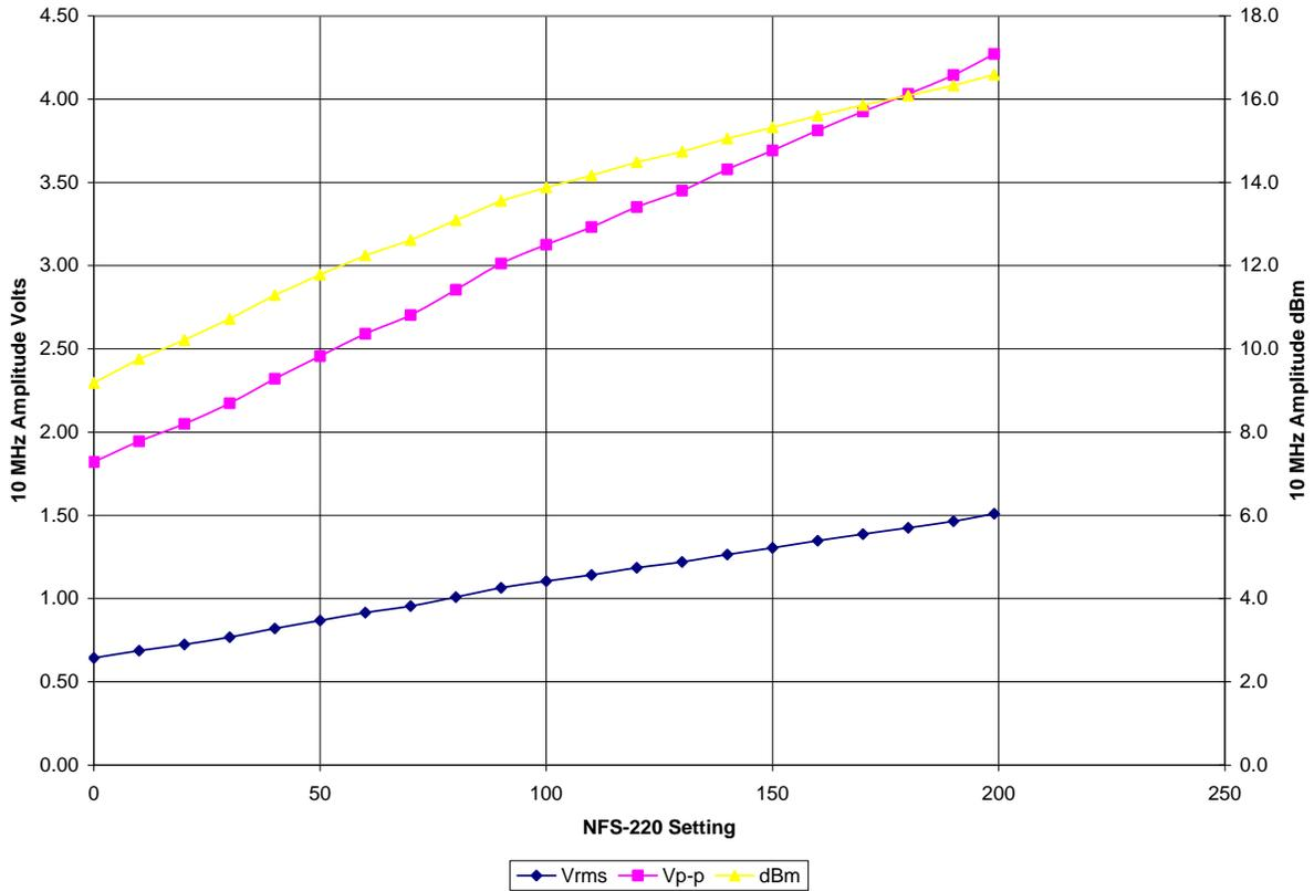
Figure 17 Setting NFS-220 10 MHz output level
