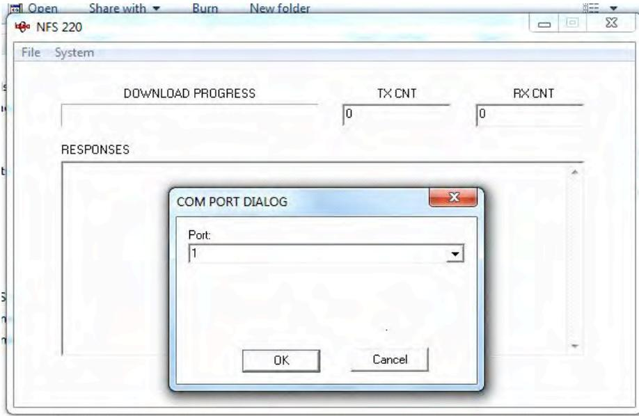
2. Connect a Null Serial Cable (crossed-over) from the computer's COM port to the unit's J10 (Console).
