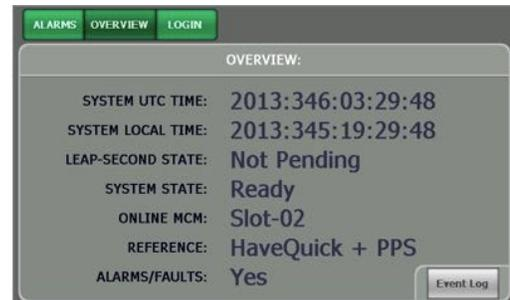
Available input reference selections include GPS (both C/A code and SAASM receivers are supported), IRIG-B, Have Quick/1PPS and external 10 MHz. In addition an MCM may be synchronized by up to 2 other MMC chassis using a fiber optic crosslink, this provides additional resiliency for the MMC time and frequency references.
