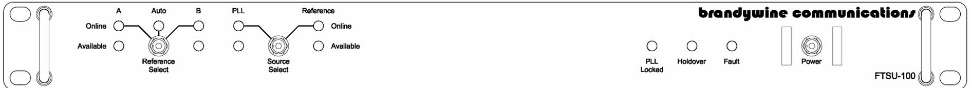
Figure 1 FTSU-100D Front Panel
